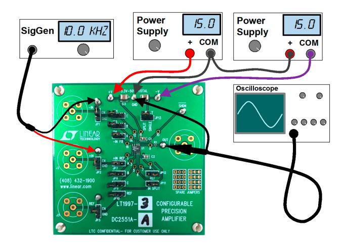
Figure 1. Proper Evaluation Equipment Setup
