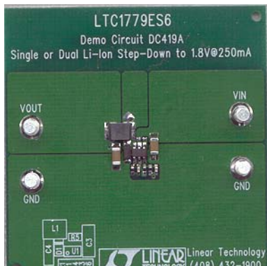
Figure 1... Quick Start connections for DC419A.
