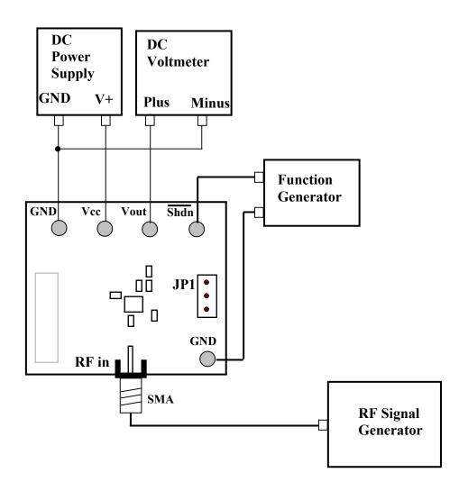
DC539A Demo Board Connection Diagram
