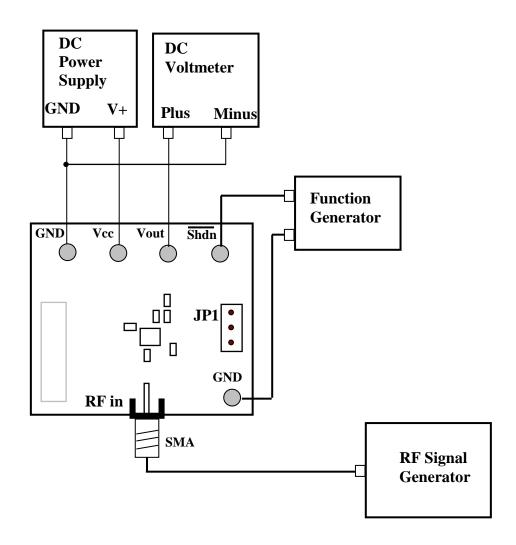
DC539B Demo Board Connection Diagram
