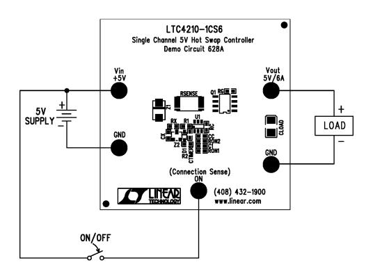
Figure 1. Proper Measurement Equipment Setup
