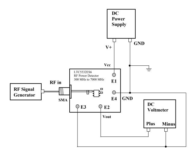
DC656A Demo Board Connection Diagram
