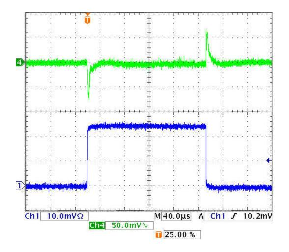
Figure 3. Load Step Response V<sub>IN</sub> = 3.3V, V<sub>OUT</sub> = 1.8V & 5A Load Step Trace 1: Output Voltage (100mV/div AC) Trace 2: Output Current (2A/div)
