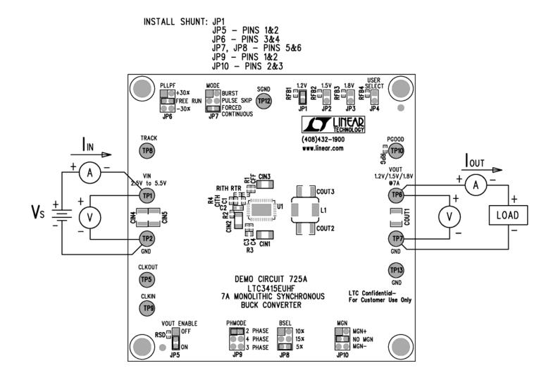
Figure 1. Proper Measurement Equipment Setup
