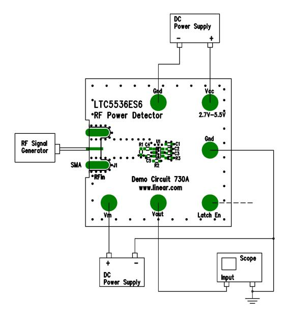
Figure 1. LTC5536 Measurements Setup
