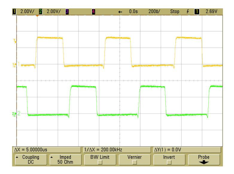
Figure 4. 180° Out-of-Phase Switching Operation
