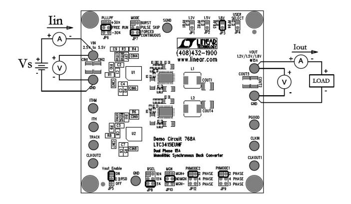
Figure 1. Proper Measurement Equipment Setup
