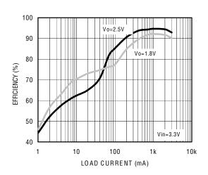
Figure 2. Efficiency vs load current (550kHz)
