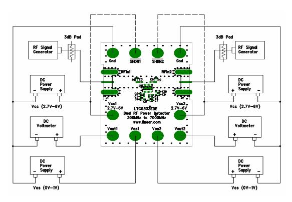
Figure 1. Proper Measurement Equipment Setup
