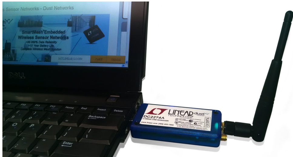
Figure 8 SmartMesh IP USB Manager (DC2274A-A) in PC
