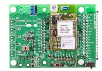
SmartMesh WirelessHART networks are populated by motes, the nodes on the network. Based on the Dust<sup>®</sup> break-through Eterna<sup>®</sup> technology, the motes are ultralow power, extending battery life to years and many times that of alternative products. In addition to extra long battery life, the motes feature an advanced array of features.
