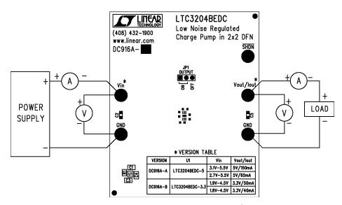
Figure 1. Proper Measurement Equipment Setup
