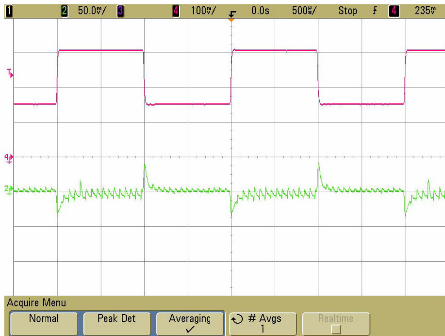
Figure 5. Transient Response Waveform at 4.2Vin and 1.5 - 3.0Aout – 500uS and 50mV / div
