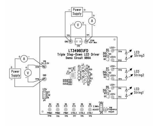
Figure 1. Proper Measurement Equipment Setup
