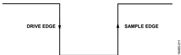
Figure 32. SPI Mode 3 SCLK Edges
