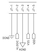
Figure 13. Schematic of Connectors to Daughter Board
