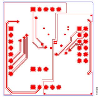
Figure 20. Layer 2 Side PCB Drawing of Daughter Board
