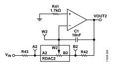
Figure 6. Linear Inverting Amplifier
