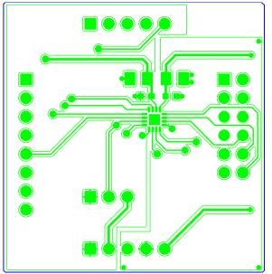
Figure 19. Component Placement Drawing of Daughter Board
