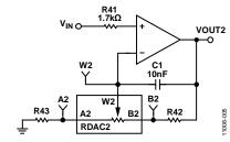
Figure 5. Pseudologarithmic Noninverting Amplifier
