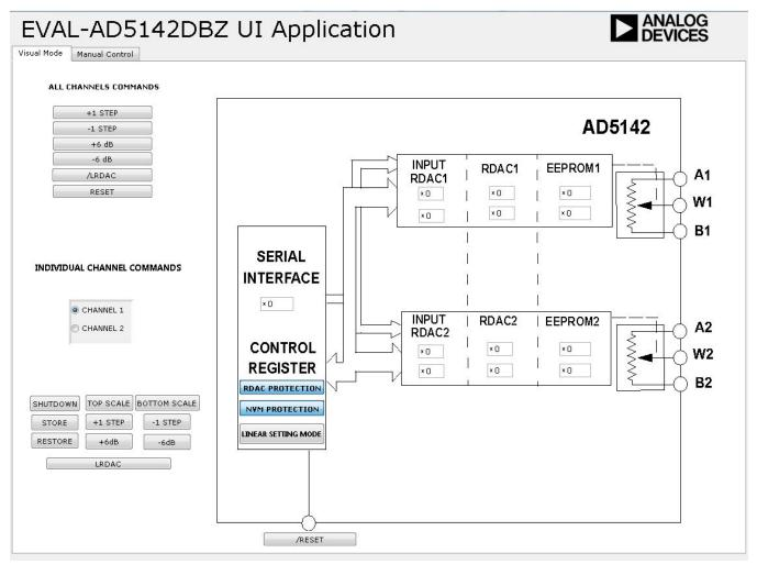
Figure 9. EVAL-AD5142DBZ Software Main Window
