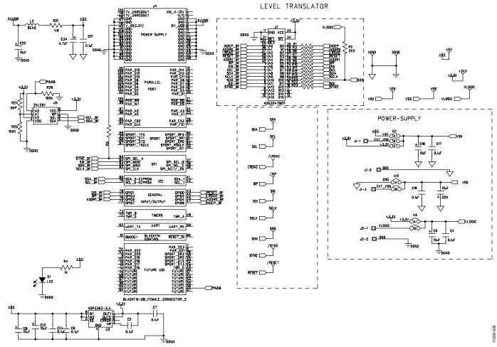
Figure 11. SDP Connector and Power Supply
