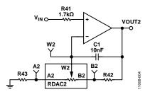
Figure 4. Linear Noninverting Amplifier
