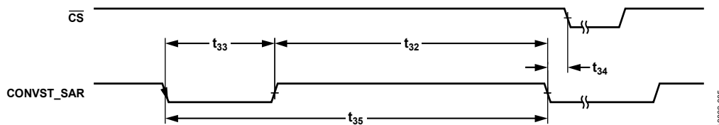
Figure 5. SAR ADC Timing Diagram
