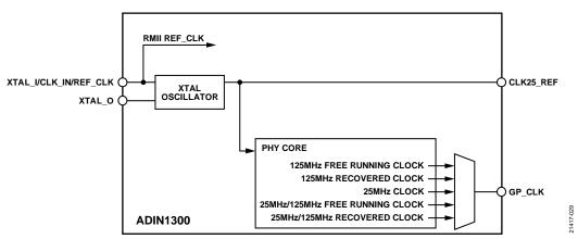
Figure 26. PHY Output Clocks Simplified Diagram
