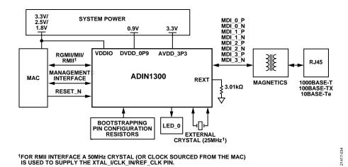
Figure 30. Simplified Typical Application Block Diagram
