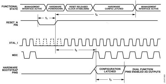
Figure 3. Hardware Reset Timing
