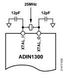
Figure 31. Crystal Oscillator Connection
