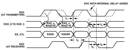
Figure 8. RGMII Receive Timing
