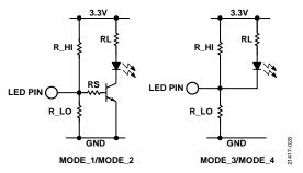
Figure 25. LED\_0 Hardware Configuration Pin Interaction
