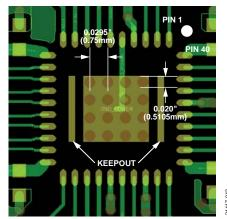
Figure 39. Exposed Paddle Via Array on EVAL-ADIN1300FMCZ
