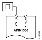
Figure 32. External Clock Connection
