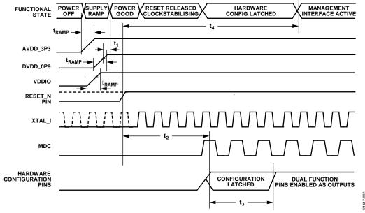
Figure 2. Power-Up Timing
