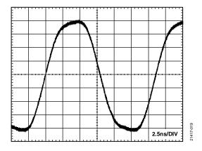
Figure 18. 1000BASE-T Test Mode 2 Output
