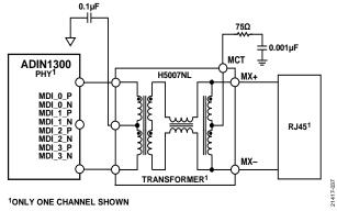
Figure 33. Isolation Using Discrete Magnetics, Only One Channel Shown, Each Channel has Separate Components to Ground
