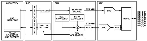
Figure 19. Simplified Channel Block Diagram
