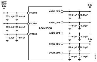
Figure 38. Supply Decoupling Overview
