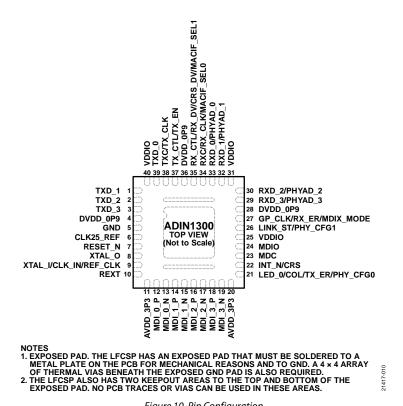
Figure 10. Pin Configuration
