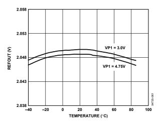
Figure 20. REFOUT vs. Temperature
