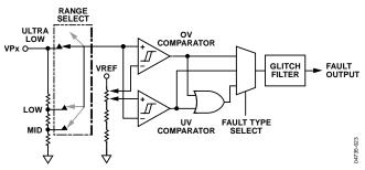
Figure 22. Supply Fault Detector Block
