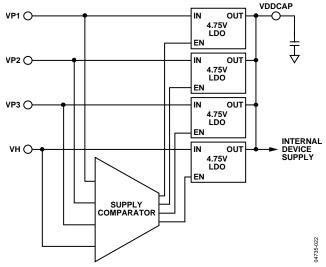
Figure 21. V<sub>DD</sub> Arbitrator Operation
