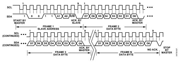
Figure 37. General SMBus Read Timing Diagram
