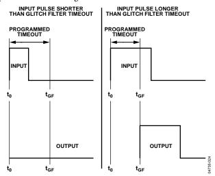
Figure 23. Input Glitch Filter Function
