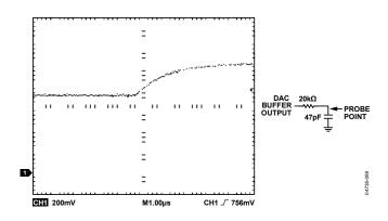
Figure 17. Transient Response of DAC Code Change into Typical Load
