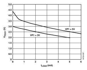
Figure 12. V<sub>PDO1</sub> (Strong Pull-Up to VPx) vs. I<sub>LOAD</sub>
