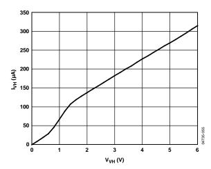
Figure 10. I<sub>VH</sub> vs. V<sub>VH</sub> (VH Not as Supply)
