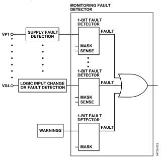
Figure 29. Monitoring Fault Detect or Block Diagram
