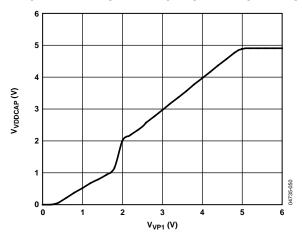
Figure 5. V<sub>VDDCAP</sub> vs. V<sub>VP1</sub>
