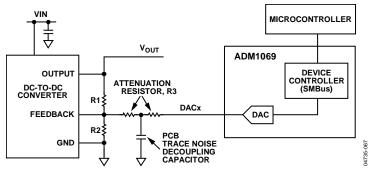
Figure 32. Open-Loop Margining System Using the ADM1069
