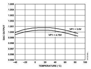
Figure 19. DAC Output vs. Temperature
