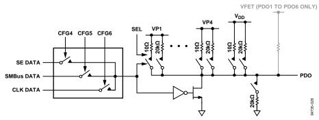
Figure 25. Programmable Driver Output
