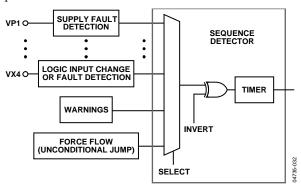
Figure 27. Sequence Detector Block Diagram
