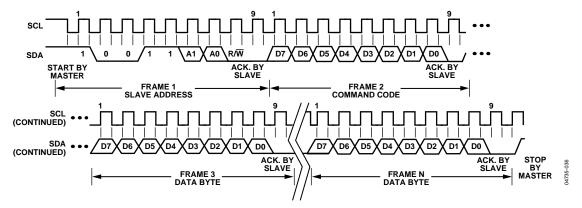
Figure 36. General SMBus Write Timing Diagram
