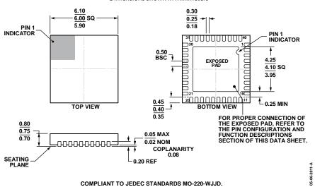
Figure 49. 40-Lead Lead Frame Chip Scale Package [LFCSP] 6 mm × 6 mm Body and 0.75 mm Package Height (CP-40-9) Dimensions shown in millimeters
