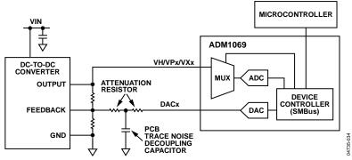
Figure 33. Closed-Loop Margining System Using the ADM1069
