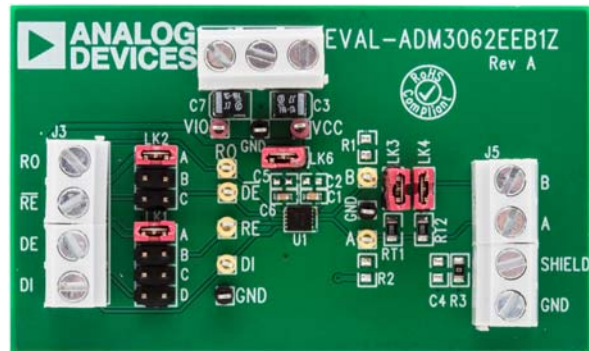
Figure 2. EVAL-ADM3062EEB1Z Evaluation Board
