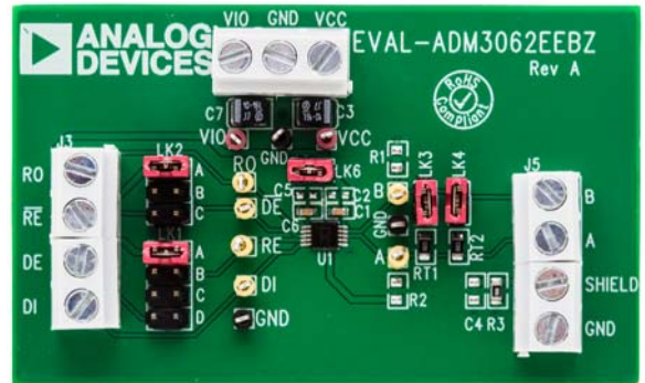
Figure 1. EVAL-ADM3062EEBZ Evaluation Board
