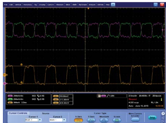
Figure 4. D_{OUT2-} and D_{OUT2+} with a 300 MHz Clock, Single-Ended and Differential
