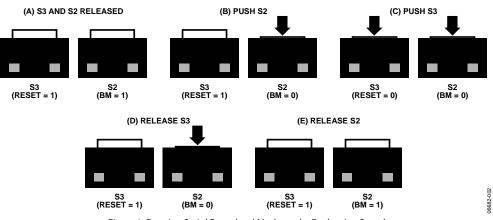
Figure 1. Entering Serial Download Mode on the Evaluation Board
