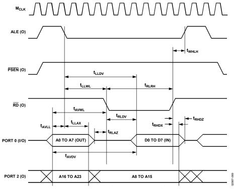
Figure 6. External Data Memory Read Cycle
