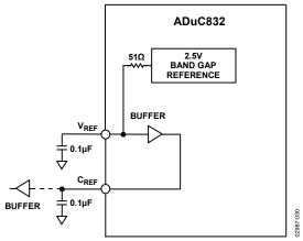
Figure 41. Decoupling VREF and CREF
