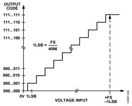
Figure 37. ADC Transfer Function
