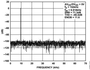
Figure 26. Dynamic Performance at  $V_{DD} = 5 V$
