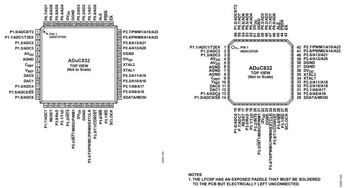
Figure 14. 52-Lead MQFP
