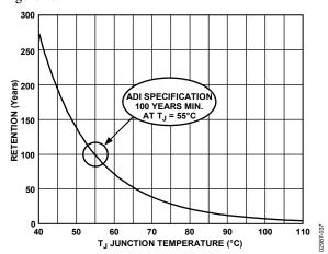
Figure 48. Flash/EE Memory Data Retention
