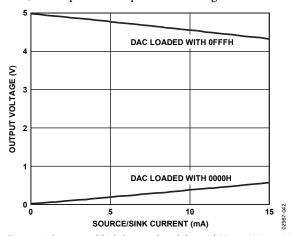
Figure 53. Source and Sink Current Capability with  $V_{REF} = AV_{DD} = 5 V$
