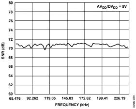
Figure 30. Typical Dynamic Performance vs. Sampling Frequency
