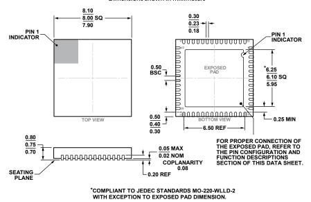
Figure 96. 56-Lead Lead Frame Chip Scale Package [LFCSP] 8 mm × 8 mm Body and 0.75 mm Package Height (CP-56-11) Dimensions shown in millimeters
