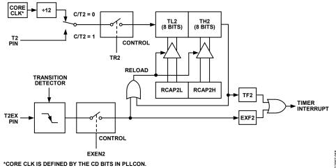
Figure 79. Timer/Counter 2, 16-Bit Autoreload Mode
