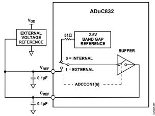
Figure 42. Using an External Voltage Reference
