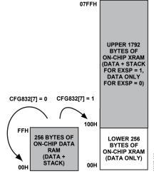
Figure 33. Extended Stack Pointer Operation
