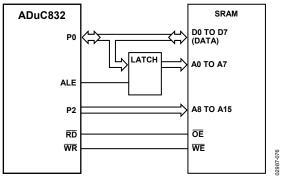
Figure 88. External Data Memory Interface (64 kB Address Space)
