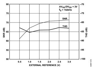
Figure 29. Typical Dynamic Performance vs.  $V_{REF}$ ,  $V_{DD} = 3 V$
