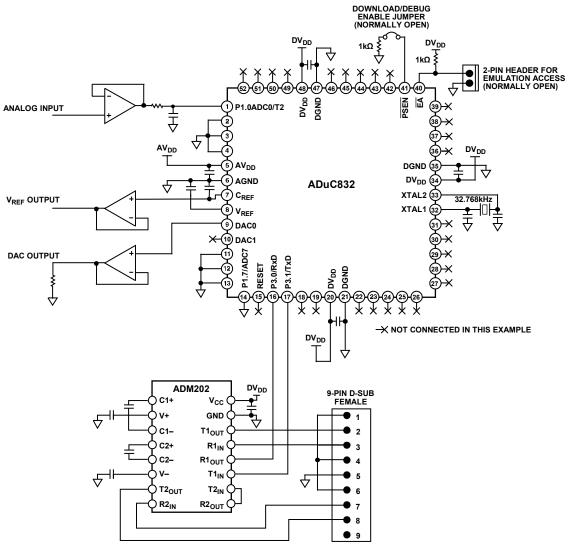
Figure 94. Example ADuC832 System (MQFP Package)
