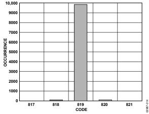
Figure 25. Code Histogram Plot,  $V_{DD} = 3 V$
