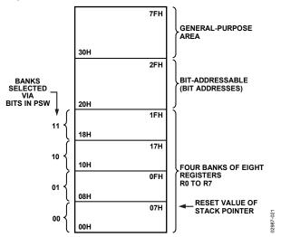
Figure 32. Lower 128 Bytes of Internal Data Memory
