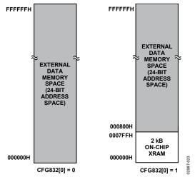
Figure 34. Internal and External XRAM
