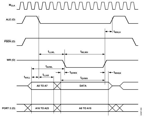
Figure 7. External Data Memory Write Cycle
