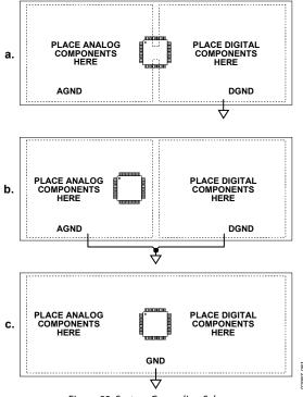
Figure 93. System Grounding Schemes
