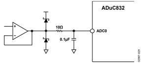
Figure 40. Buffering Analog Inputs
