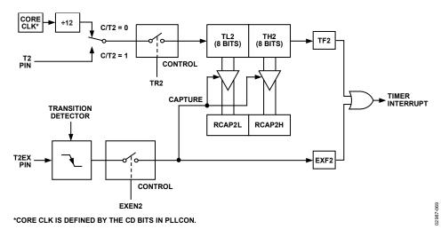
Figure 80. Timer/Counter 2, 16-Bit Capture Mode Rev. C | Page 74 of 92
