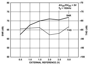
Figure 28. Typical Dynamic Performance vs.  $V_{REF}$ ,  $V_{DD} = 5 V$
