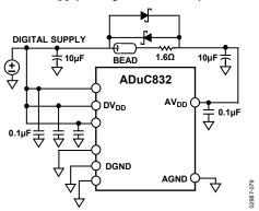
Figure 91. External Single-Supply Connections
