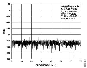
Figure 27. Dynamic Performance at  $V_{DD} = 3 V$
