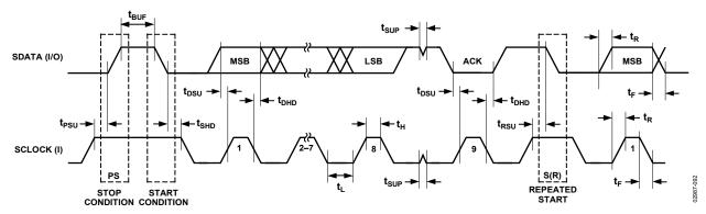
Figure 9. I<sup>2</sup>C Compatible Interface Timing
