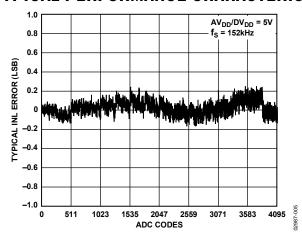
Figure 16. Typical INL Error,  $V_{DD} = 5 V$
