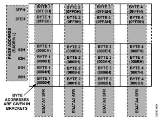
Figure 50. Flash/EE Data Memory Control and Configuration
