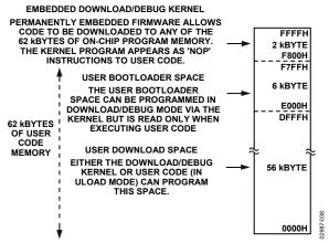
Figure 49. Flash/EE Program Memory Map in ULOAD Mode
