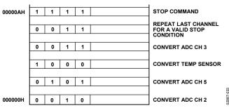
Figure 44. Typical DMA External Memory Preconfiguration
