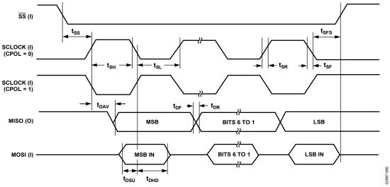
Figure 12. SPI Slave Mode Timing (CPHA = 1)
