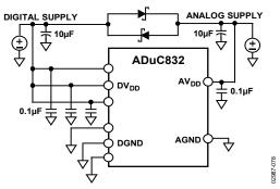
Figure 90. External Dual-Supply Connections
