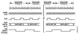
Figure 81. UART Serial Port Transmission, Mode 0
