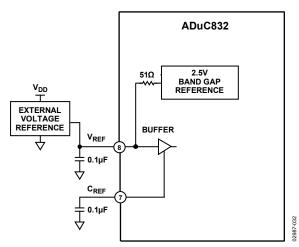
Figure 43. Using an External Voltage Reference
