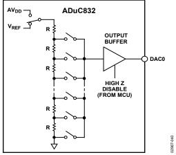
Figure 51. Resistor String DAC Functional Equivalent
