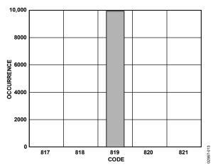
Figure 24. Code Histogram Plot,  $V_{DD} = 5 V$
