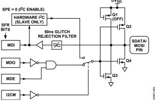
Figure 74. SDATA/MOSI Pin I/O Functional Equivalent in I<sup>2</sup>C Mode
