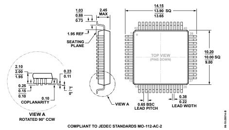
Figure 95. 52-Lead Metric Quad Flat Package [MQFP] (S-52-2) Dimensions shown in millimeters
