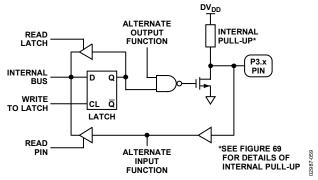
Figure 70. Port 3 Bit Latch and I/O Buffer
