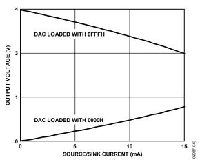
Figure 54. Source and Sink Current Capability with  $V_{REF} = AV_{DD} = 3 V$
