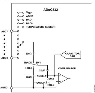
Figure 39. Internal ADC Structure
