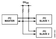
Figure 64. Typical I<sup>2</sup>C System
