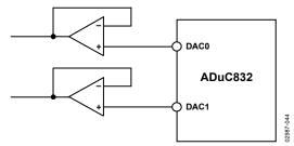
Figure 55. Buffering the DAC Outputs
