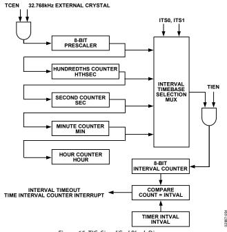
Figure 65. TIC, Simplified Block Diagram
