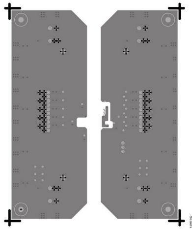
Figure 7. GND1 and GND2 Planes (Layer 3)
