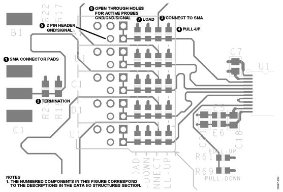
Figure 3. Configuration and Monitoring Structures
