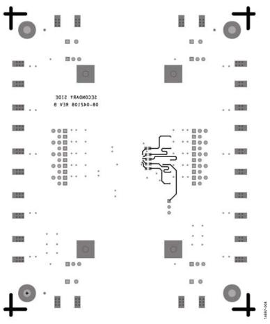
Figure 8. Bottom Layer Assembly and Routing (Layer4)
