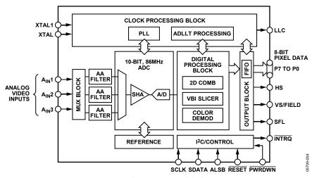
Figure 4. 40-Lead LFCSP Functional Block Diagram
