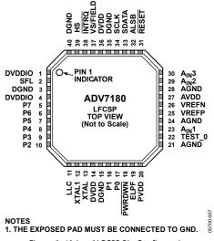
Figure 9. 40-Lead LFCSP Pin Configuration
