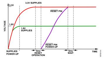
Figure 13. Power-Up Sequence of the 32-Lead LFCSP
