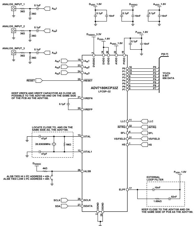
Figure 60. 32-Lead LFCSP Typical Connection Diagram
