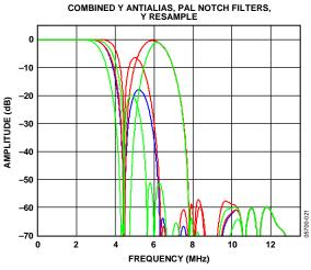
Figure 26. Combined Y Antialias, PAL Notch Filters
