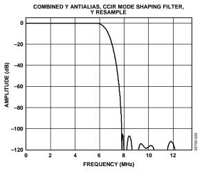
Figure 25. Combined Y Antialias, CCIR Mode Shaping Filter
