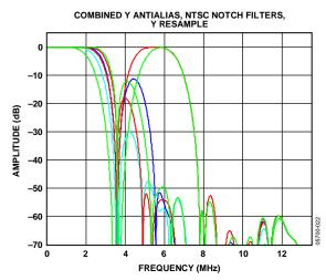
Figure 27. Combined Y Antialias Filter, NTSC Notch Filters
