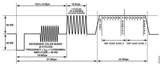
Figure 50. CCAP Waveform and Decoded Data Correlation
