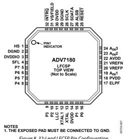
Figure 8. 32-Lead LFCSP Pin Configuration
