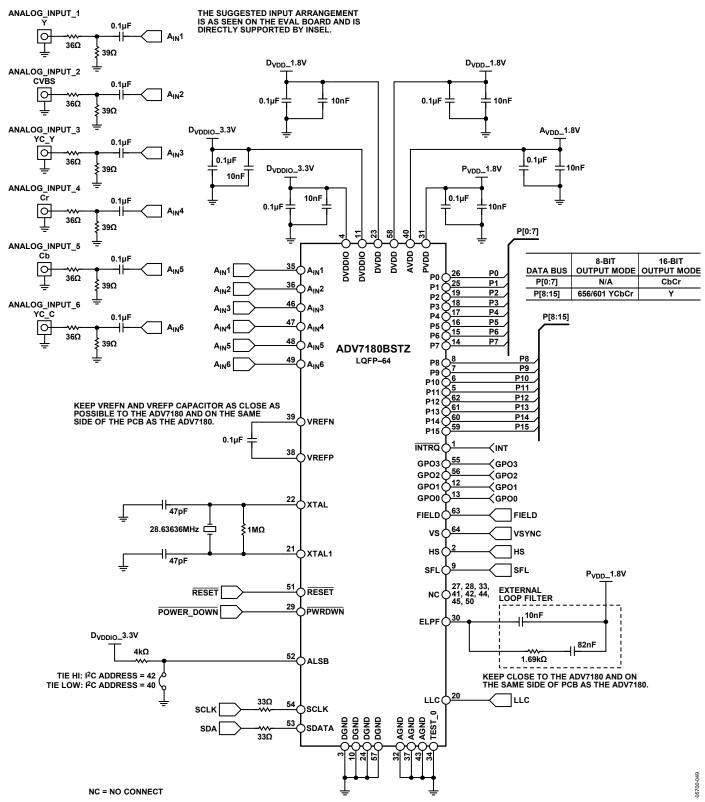
Figure 58. 64-Lead LQFP Typical Connection Diagram
