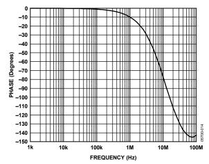
Figure 19. Antialiasing Filter Phase Response
