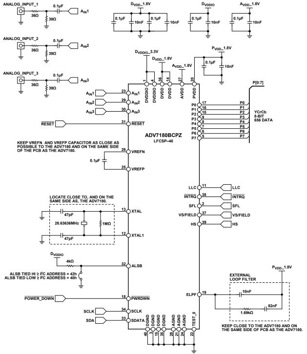
Figure 57. 40-Lead LFCSP Typical Connection Diagram
