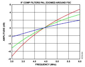
Figure 35. PAL IF Filter Compensation
