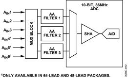
Figure 17. Antialias Filter Configuration
