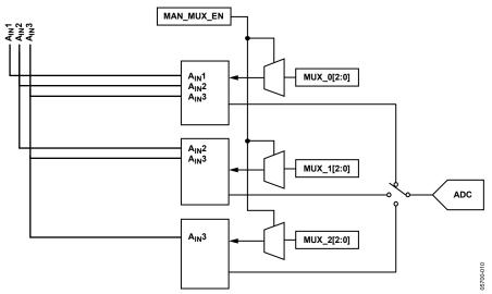
Figure 15. 40-Lead and 32-Lead LFCSP Internal Pin Connections
