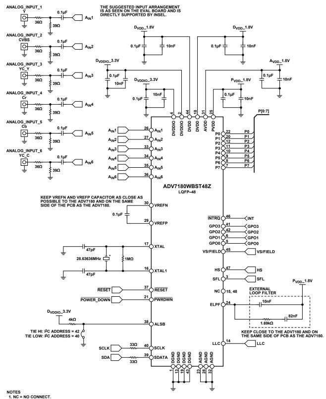
\*REFER TO ANALOG DEVICES CRYSTAL APPLICATION NOTE FOR PROPER CAPACITOR LOADING
