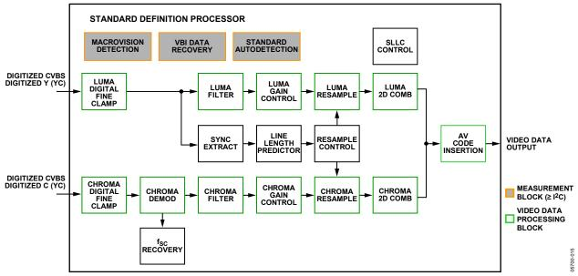
Figure 20. Block Diagram of the Video Processor
