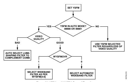
Figure 23. YSFM and WYSFM Control Flowchart
