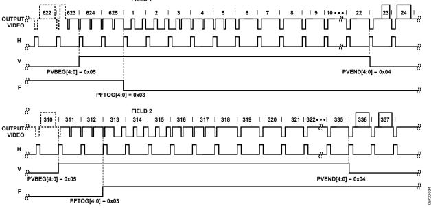
Figure 43. PAL Default, ITU-R BT.656 (the Polarity of H, V, and F Is Embedded in the Data)
