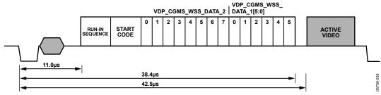
Figure 48. WSS Waveform
