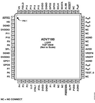
Figure 10. 64-Lead LQFP Pin Configuration
