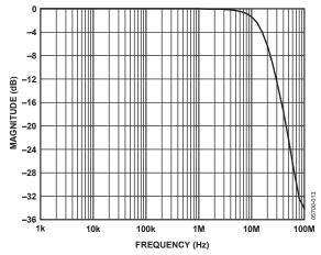
Figure 18. Antialiasing Filter Magnitude Response
