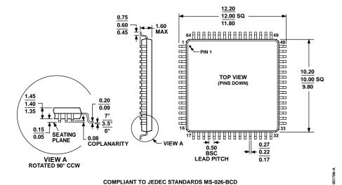
Figure 63. 64-Lead Low Profile Quad Flat Package [LQFP] 10 mm × 10 mm Body (ST-64-2) Dimensions shown in millimeters
