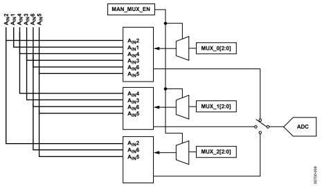
Figure 14. 64-Lead and 48-Lead LQFP Internal Pin Connections
