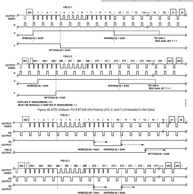
Figure 39. NTSC Typical VSYNC/FIELD Positions Using the Register Writes in Table 65
