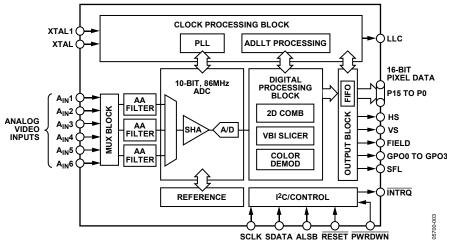
Figure 3. 64-Lead LQFP Functional Block Diagram
