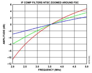
Figure 34. NTSC IF Filter Compensation
