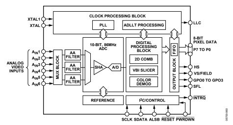
Figure 5. 48-Lead LQFP Functional Block Diagram
