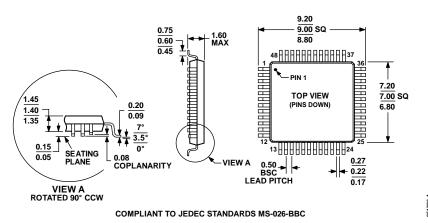
Figure 64. 48-Lead Low Profile Quad Flat Package [LQFP]
