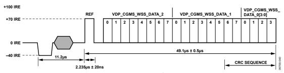
Figure 49. CGMS Waveform
