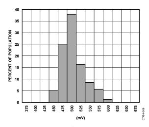
Figure 9. ST2 Output Change at 25°C ( $V_{RATIO} = 5 V$ )
