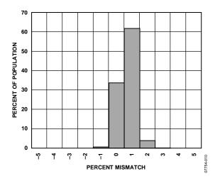
Figure 10. Self-Test Mismatch at  $25^{\circ}$ C ( $V_{RATIO} = 5 V$ )
