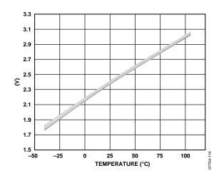
Figure 14.  $V_{TEMP}$  Output over Temperature, 256 Parts ( $V_{RATIO} = 5 V$ )
