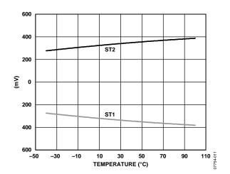
Figure 11. Typical Self-Test Change over Temperature
