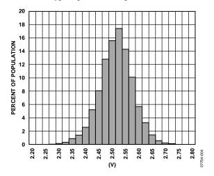
Figure 4. Null Output at  $25^{\circ}$ C ( $V_{RATIO} = 5 V$ )
