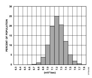
Figure 6. Sensitivity at  $25^{\circ}$ C ( $V_{RATIO} = 5 V$ )
