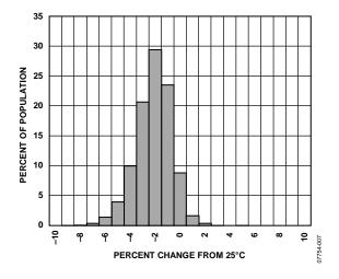
Figure 7. Sensitivity Drift over Temperature
