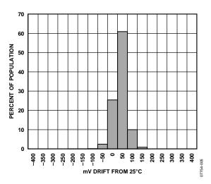
Figure 5. Null Drift over Temperature ( $V_{RATIO} = 5 V$ )
