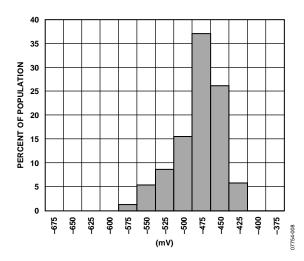
Figure 8. ST1 Output Change at 25°C ( $V_{RATIO} = 5 V$ )
