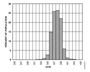
Figure 12. Current Consumption at 25°C ( $V_{RATIO} = 5 V$ )
