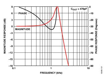
Figure 15. ADXRS646-EP Frequency Response with a 2.2 kHz Output Filter
