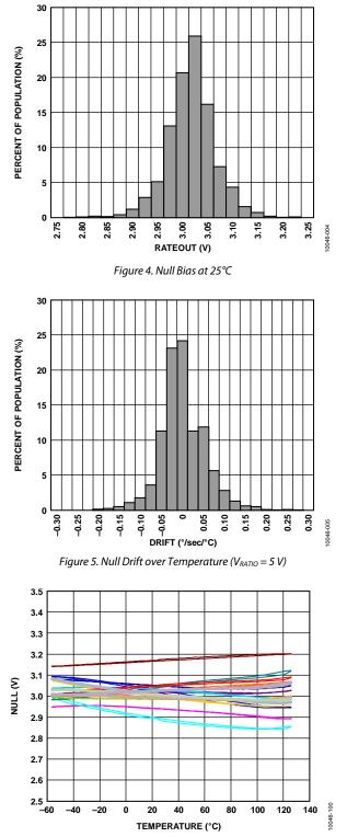
Figure 6. Null Output over Temperature, 16 Parts in Sockets (V<sub>RATIO</sub> = 5 V)
