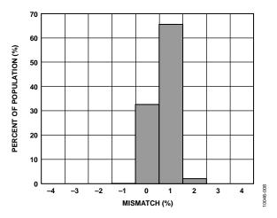
Figure 12. Self-Test Mismatch at  $25^{\circ}C$  ( $V_{RATIO} = 5 V$ )
