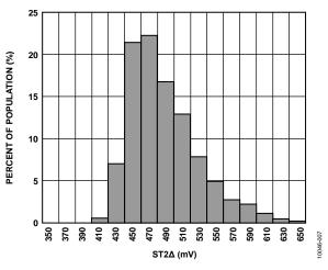
Figure 13. ST2 Output Change at  $25^{\circ}C$  (V<sub>RATIO</sub> = 5 V)
