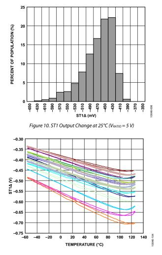
Figure 11. ST1 Output Change vs. Temperature, 16 Parts in Sockets
