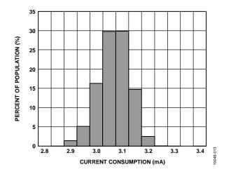
Figure 18. Current Consumption at  $25^{\circ}C$  (V<sub>RATIO</sub> = 5 V)
