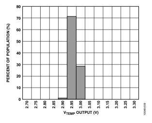
Figure 16.  $V_{TEMP}$  Output at 25°C ( $V_{RATIO} = 5 V$ )
