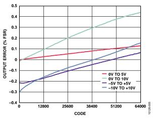
Figure 5. Measured Error (% FSR) for Voltage Output Ranges
