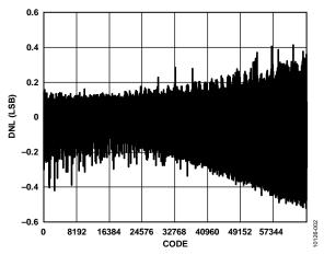
Figure 2. Measured DNL of Circuit for ±10 V Output Range
