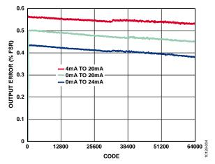
Figure 4. Measured Error (% FSR) For Current Output Ranges
