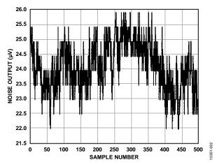
Figure 2. Noise Output (V<sub>REF</sub> = 4.096 V, AV<sub>DD</sub> = 5 V, Output Data Rate = 4.7 Hz, Gain = 1, Chop Disabled, SINC4 Filter)
