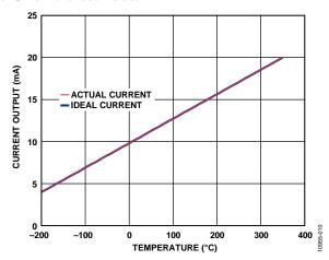
Figure 12. Temperature in  $^{\circ}$ C vs. Current out in mA (Blue = Ideal Value, Closed-Loop Operation: DAC Output Compensated by ADC0 Measurement
