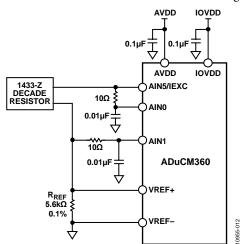
Figure 14. Test Setup for Measuring RTD Error
