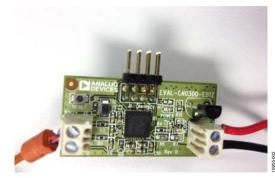
Figure 2. EVAL-CN0300-EB1Z Board Used for this Circuit
