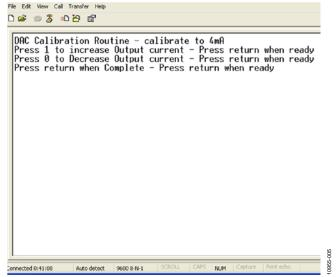
Figure 7. Output of HyperTerminal when Calibrating the DAC
