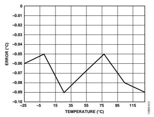
Figure 15. Error in °C of RTD Measurement Using Piecewise Linearization Code and ADCO Measurements
