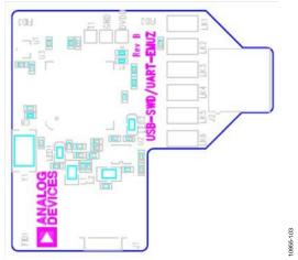
Figure 4. Analog Devices J-Link OB Emulator Top View
