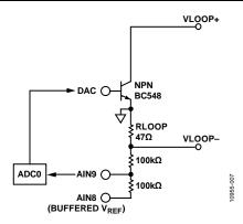
Figure 9. Closed-Loop Control 4 mA to 20 mA DAC Output
