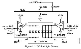
Each half of the AD8592 op amp acts as a 60 mA current source to supply the LCD backlight currents. The AD8592 can source and sink up to 250 mA, and the 100 nF capacitor ensures a soft startup.
