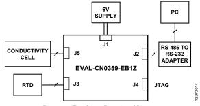
Figure 14. Test Setup Functional Diagram
