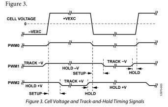
The output of the AD8253 in amp (U15) drives two parallel track-and-hold circuits composed of ADG1211 switches (U17A/U17B), series resistors (R34/R36), hold capacitors (C50/C73), and unity-gain buffers (U10/U13).
