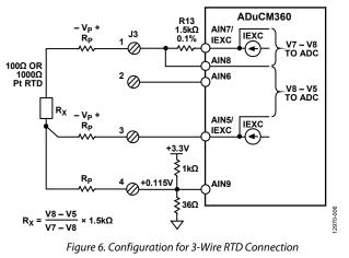
The second matched IEXC current source (AIN5/IEXC) develops a voltage across the lead resistance in series with Terminal 3 that cancels the voltage dropped across the lead resistance in series with Terminal 1. The measured V8 – V5 voltage is therefore free of lead resistance error.
