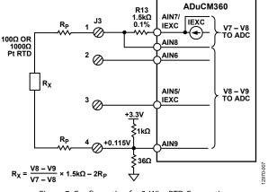
Figure 7. Configuration for 2-Wire RTD Connection
