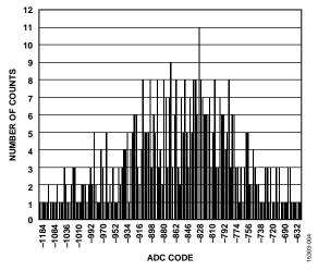
Figure 4. Shorted Input Histogram For Single Channel , 512 Samples, ADC Sinc3 Filter On, Chop Enabled, 50 Hz Data Rate
