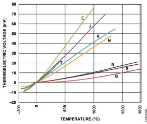
Figure 3. Thermocouple Output Voltage vs. Temperature
