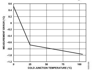
Figure 8. EVAL-CN0394-ARDZ Temperature Measurement Error for Type J Thermocouple at Room Temperature for Cold Junction Temperatures of  $0^{\circ}$ C,  $25^{\circ}$ C, and  $105^{\circ}$ C
