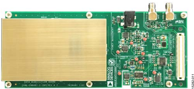
Figure 12. EVAL-CN0407-SDPZ Photograph (with Shield Installed)
