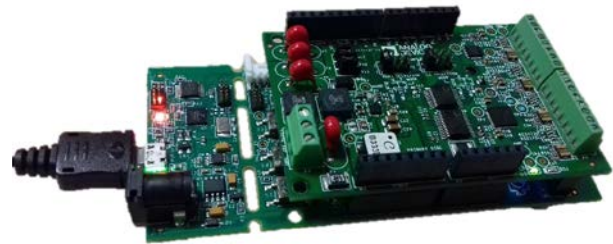
Figure 13. EVAL-CN0414-ARDZ Connected to EVAL-ADICUP3029
