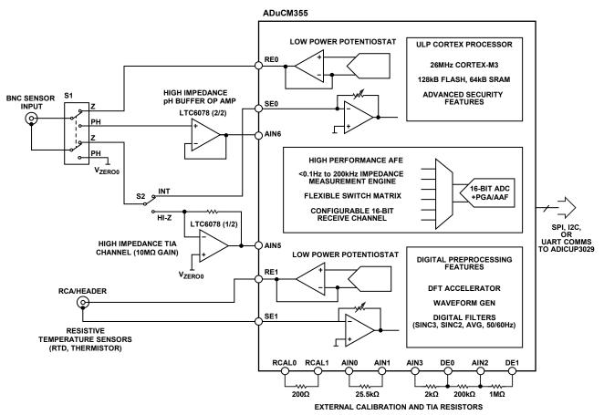
Figure 1. Simplified Circuit Block Diagram
