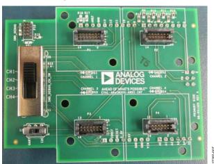
Figure 7. EVAL-M355-ARDZ-INT Arduino Shield Board
