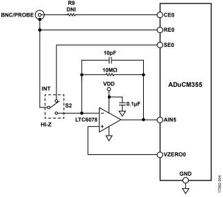
Figure 4. Schematic for Conductivity Measurement
