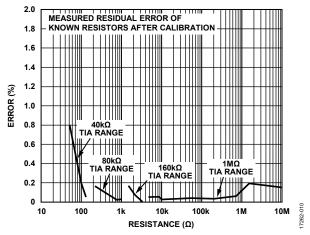
Figure 10. Resistor Measurement Calibration Result
