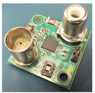
Figure 5. EVAL-CN0428-EBZ Water Sensor Boards
