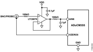
Figure 2. Schematic for pH Measurement
