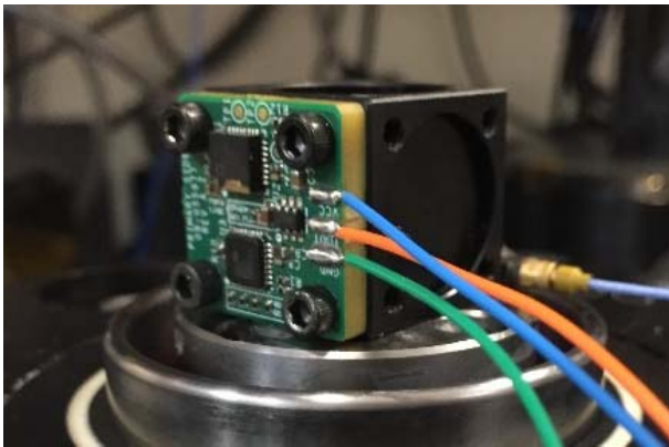
Figure 3. EVAL-CN0533-EBZ Attached to a Shaker Table Using the EVAL-XLMOUNT1
