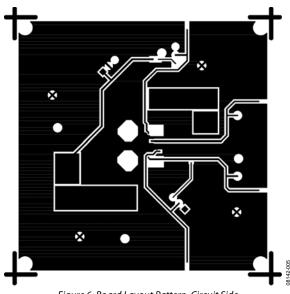
Figure 6. Board Layout Pattern, Circuit Side
