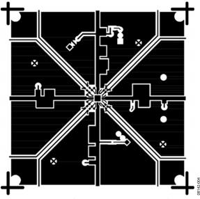
Figure 4. Board Layout Pattern, Component Side
