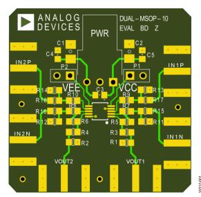
Figure 1. Evaluation Board, Component Side
