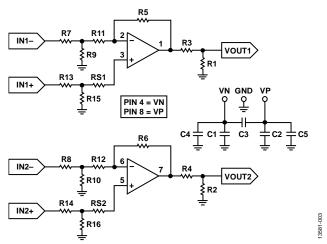
Figure 3. 8-Lead MSOP Evaluation Board Schematic
