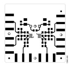
Figure 5. Component Side Layout Pattern
