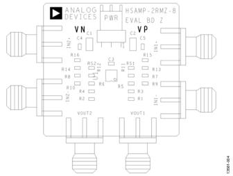
Figure 4. Component Side Assembly Drawing
