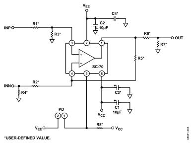
Figure 3. Evaluation Board Schematic
