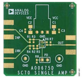
Figure 1. Component Side of Evaluation Board
