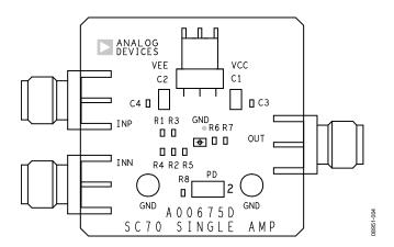
Figure 4. Component Side Assembly Drawing
