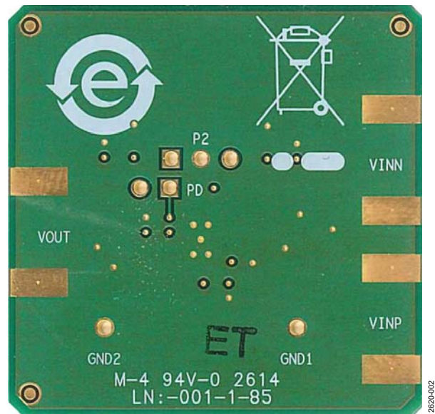
Figure 2. SO8 SINGLE AMP Evaluation Board, Secondary Side
