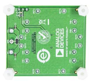
Figure 2. EVAL-LTC2065-TQFN, Secondary Side
