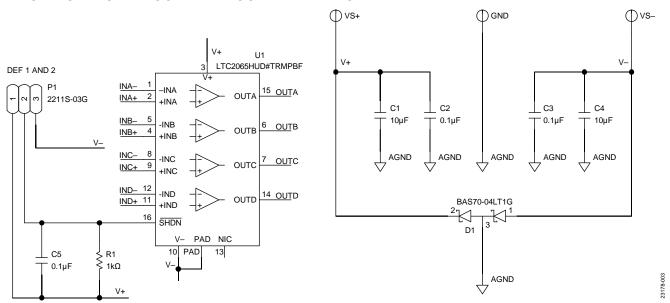
Figure 3. EVAL-LTC2065-TQFN Schematic, Page 1
