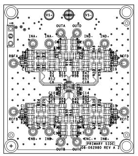
Figure 5. EVAL-LTC2065-TQFN Layout Pattern, Primary Side
