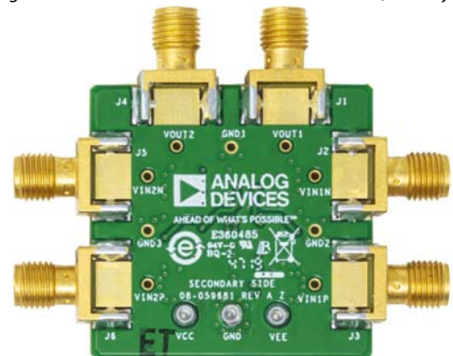
Figure 2. EVAL-LTC6227MS8E/EVAL-LTC6229MS8E, Secondary Side
