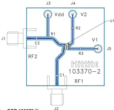
\* R2 = R3 = 100 Ohm. These resistors are optional and may be used to enhance decoupling of the RF path from the control inputs.
