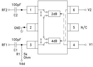
DC blocking capacitors C1 & C2 are required on RF1 & RF2. Choose C1 = C2 =  $100 \sim 300$  pF to allow lowest customer specific frequency to pass with minimal loss. R1 = 5K Ohm is required to supply voltage to the circuit through either PIN 3 or PIN 1.
