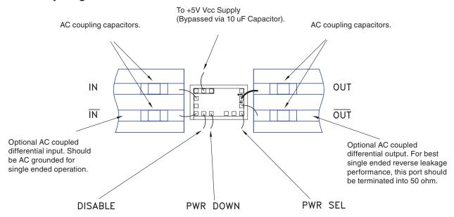
This port should be grounded for normal operation. Applying +5V to this port will disable the input buffer amplifier. This port should be grounded for normal operation. Applying +5V to this port will power down the device.
