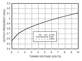
Sensitivity vs. Tuning Voltage, Vcc= +3V
