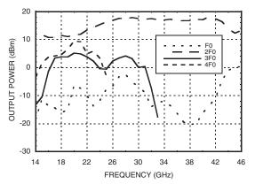
GaAs MMIC x2 ACTIVE FREQUENCY MULTIPLIER, 22 - 46 GHz OUTPUT
