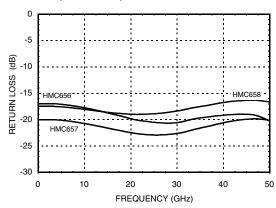
[1] Data taken with die mounted to plate and RF probed through two 1 mil diameter wire bonds.
