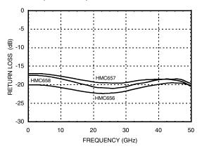
[2] Data taken with die mounted to plate and RF probed through two 3 x 0.5 mil ribbon bonds.
